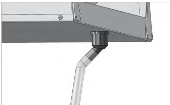
Fig. 4. Slide the provided drain hose onto the drain nozzle.
