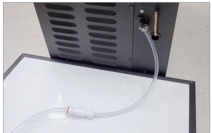
FIG. 5. Installed check valve.
