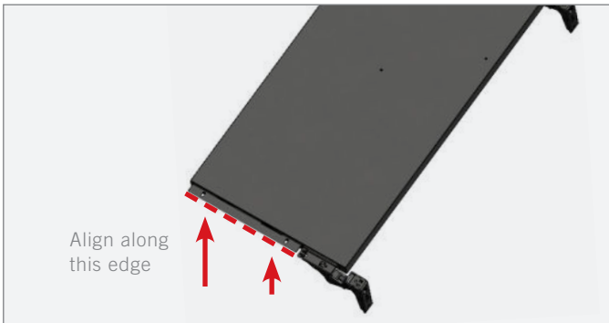
FIG. 3. Align along the bottom door bracket edge. Front of door assembly shown.
