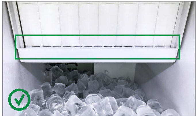
CORRECT. Ice guide finger holes are hidden; ice guide slotted holes are visible.
