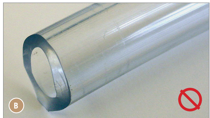
FIG. 4. A: Correct, square cut; B: Incorrect, jagged cut.
