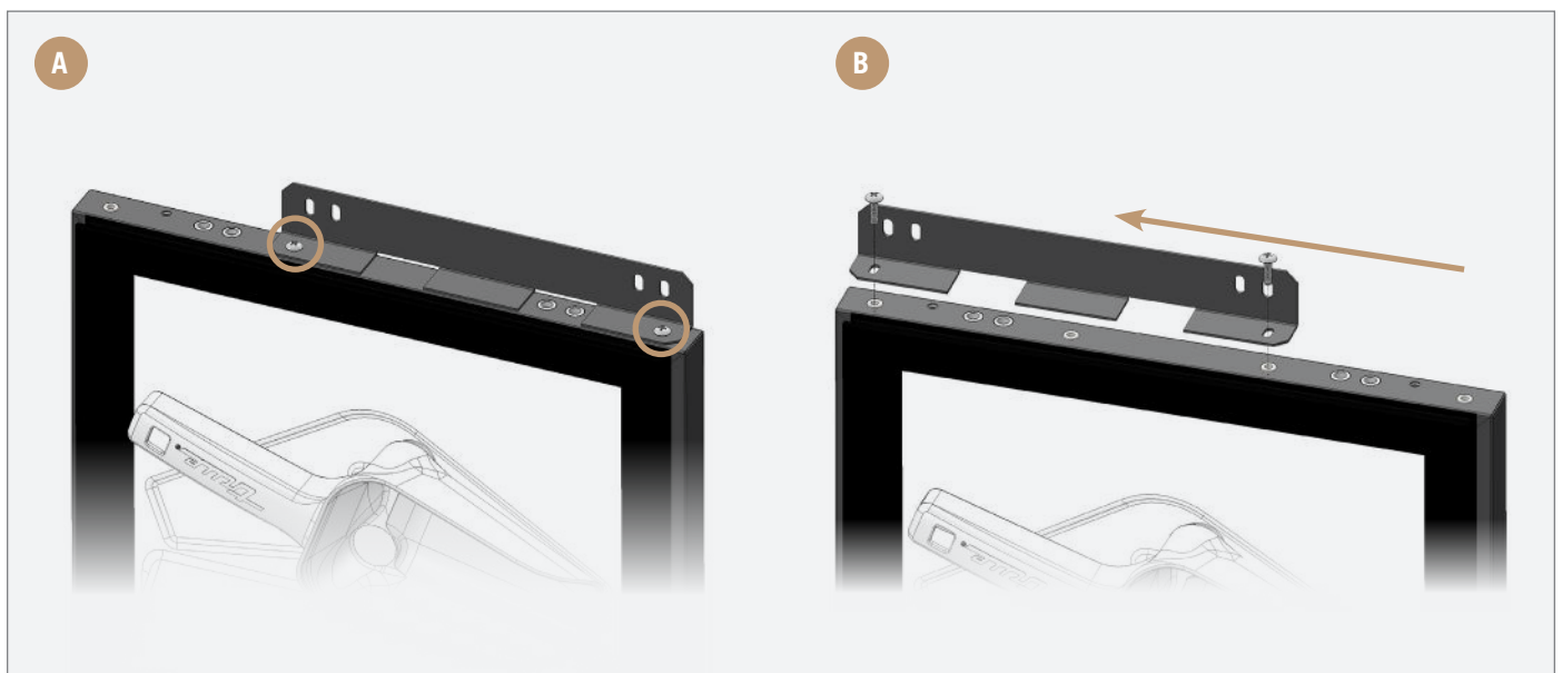
FIG. 5. Top Bracket shown. A: Door Skin bracket screw locations. B: Move the door skin bracket to the opposite side.
