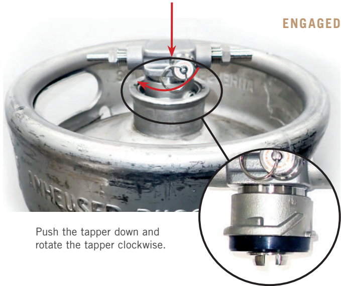
FIG. 10. Installed and connected taper. Be sure the hose clamps are tightened to prevent leaks.
