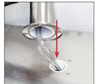
FIG. 2. Thread the draft standard lines into the cabinet.
