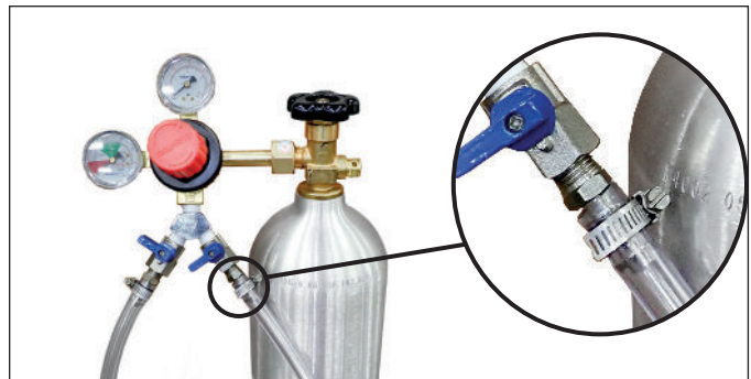
FIG. 7. Installed pressure regulator and air hoses. Be sure the hose clamps are tightened to prevent leaks.
