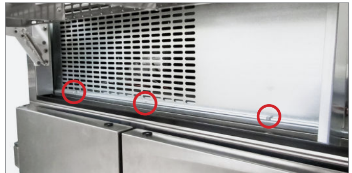
Fig. 9. Rainshield screw locations.
