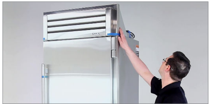
Fig. 2. Inspect the unit's exterior for visible damage.
