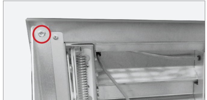
Fig. 8. Bracket screw location. Other bracket not shown.
