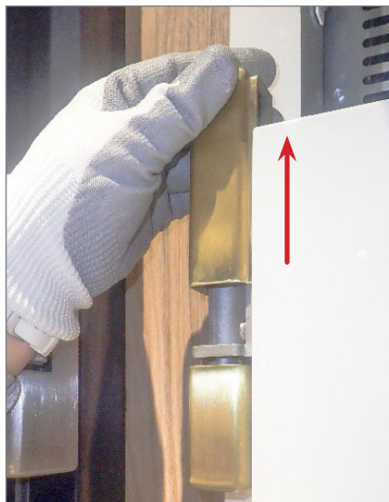
Fig. 2. Remove the hinge covers.
